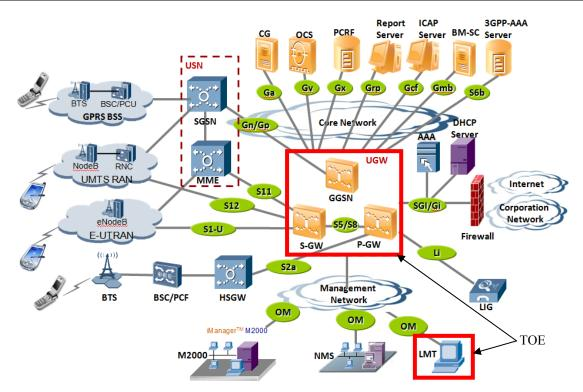
Figure 1 TOE and its environment
